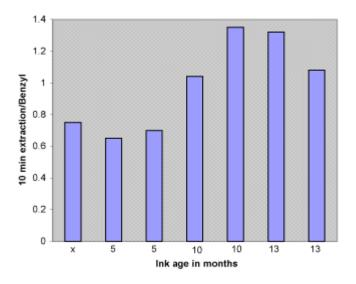
Experiment 4- R-Ratios on a Papermate Black Ball Point Ink Known dated inks written in 1992, 1993, 1994 and 1995 on bond paper were analyzed using the R-Ratio method. **Graph 4 below** shows the results that all of these inks were distinguishable as to age. Note the 3 minute extraction time is missing for the 1992 sample, because the pipette was dropped.
